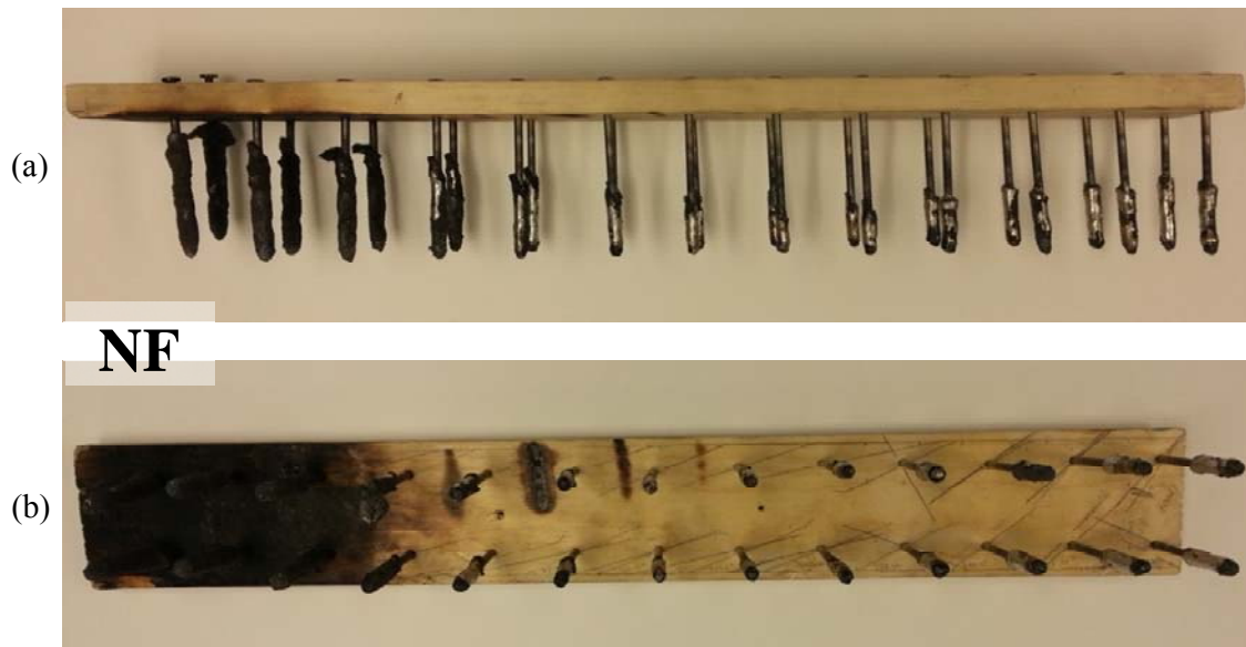
Figure 20- Pictures of one of the nail board used for the measurements at the commercial steel caster (a) front view and (b) bottom view
